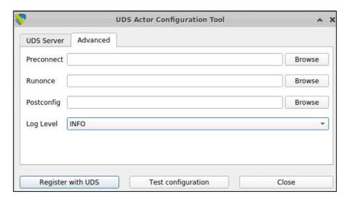
It is very important to bear in mind that to apply the values of the "Advanced" tab, it will always be necessary to carry out the registration process afterwards. If you add any script or modify the log level and you have not registered the Actor again, these will not apply.
