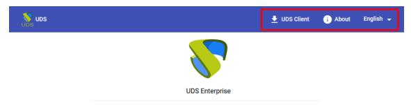
In order to add links to the top bar of the home page, enter the UDS Server (Using WinSCP or similar software) and access the index.html file in the path /var/ server/uds/templates/uds/modern/index.html and in the line where it says <body>replace it with the following code:
