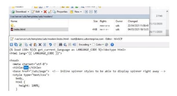
Once the text has been modified, it is necessary to restart the UDS Server Appliance for the change to take effect.
