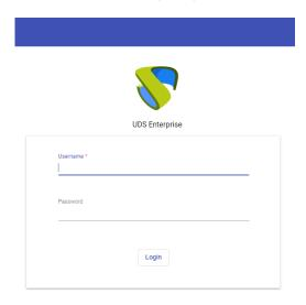
To add text below the login portal form, enter the tag "login-container :: after" in the "css" field. With HTML code you will indicate the position where you want to place it within the footer. Example:
