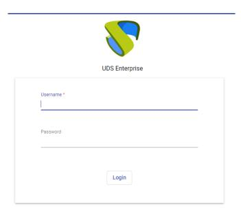
If you have modified the size of the upper bar, you must modify the position of both the logo and the form on the login screen. In order to modify the positioning of the login image, in the event that the upper bar overlaps, you must enter the label "login-brand" in the "css" field. With HTML code you can indicate the position where you want to place it. Example:
