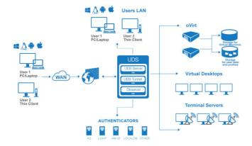
Through these very intuitive instructions, the UDS Enterprise components are hosted on the oVirt platform on which the virtual desktops are going to be deployed.
