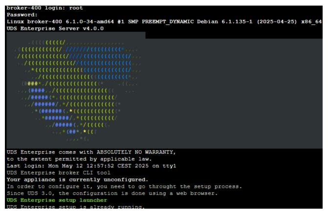
If the server has not been assigned an IP address automatically, we must do it through the command: **uds ip**
