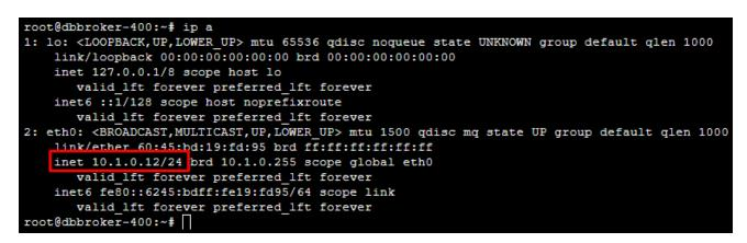
Once we confirm that we have network connectivity, we will proceed to configure the UDS Server component (If a DHCP server is not available on the network, a fixed IP address must be indicated in the /etc/network/interfaces file).
