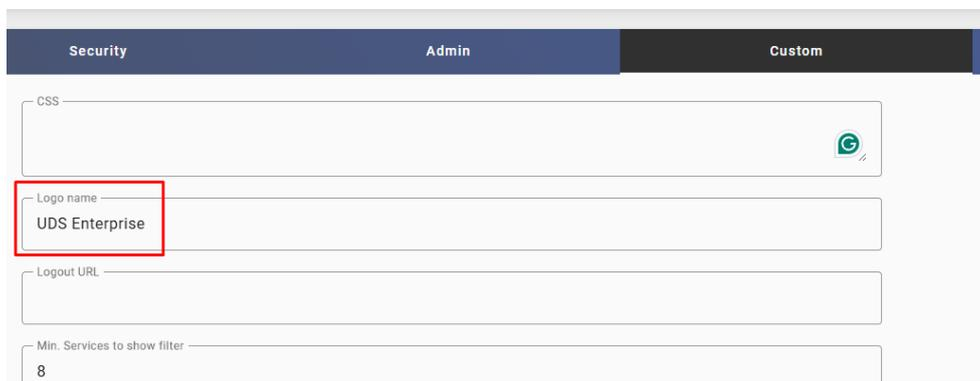
For this modification to be applied, we must press the "save" button and restart the Appliance UDS Server (or the "udsweb" service).
